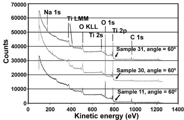
Fig. 6. XPS survey spectra for the surface of TiO<sub>2</sub> films prepared from the precursors A and B.
