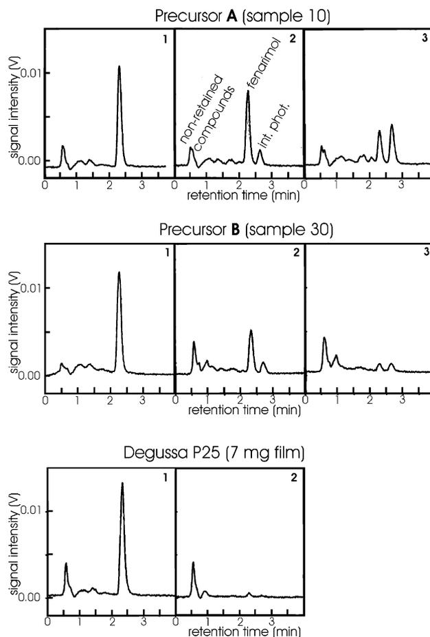
Fig. 9. Chromatograms of Fenarimol (5 mg/L aqueous solution) degradation for three TiO<sub>2</sub> thin films samples, after 1 and 3 h of UV irradiation. Notes for this figure: 1—Initial time; 2—After 1 h of irradiation; 3—After 3 h of irradiation.
