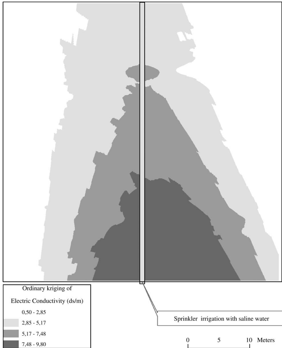
Fig. 2. Soil electrical conductivity (1:2) map of the field cultivated with lettuce and irrigated with saline water after ordinary kriging, showing a not perfect gradient around irrigation line.
