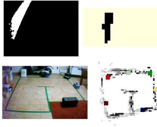
Figure 7: Examples of memory maps. Top-left: binary image (tilt T1) with segmented green tape. Top-right: resulting  $(x,y)$  Cartesian STM map when looking forward. Bottom: picture of the robot’s sandbox and a built LTM map after completing a SLAM task. Reference objects are marked by colored squares.
