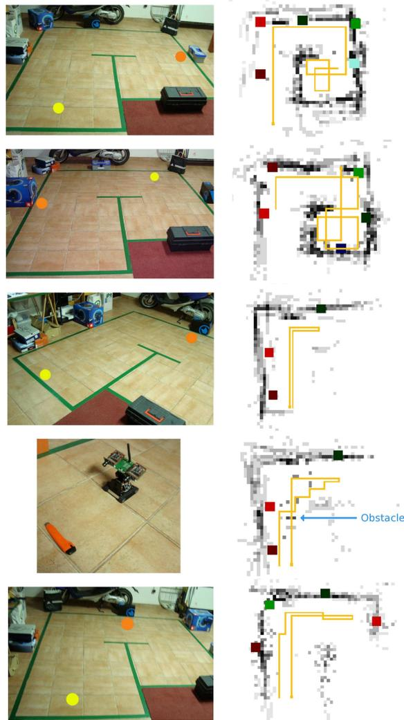
Figure 8: Top to bottom: results of tests 1 to 5. The yellow dots in the pictures are starting points, the orange dots are target objects. The robot's trajectory is shown by orange lines in the maps.
