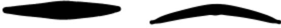
Figure 2. The contour perimeter/convex hull perimeter ratios of these two contours are equal but the area ratio is different.
