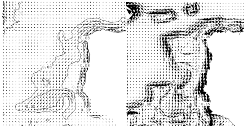
Figure 3: Velocities obtained with cartesian (left) and double sigma (right) coordinates at 400 m depth.
