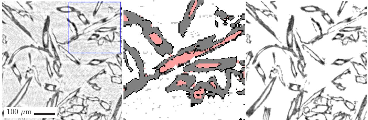
**Figure 2.** Result of the noise removal stage shown on a representative slice. *Left:* Original data with marked ROI. *Middle:* Thresholding process; cell wall voxels  $\geq t_{\text{high}}$  (dark gray), additional neighbored voxels  $\geq t_{\text{low}}$  (black), small regions of noise voxels  $\geq t_{\text{high}}$  (light gray.) The light red regions inside the fiber walls represent the fiber lumen. *Right:* Data after noise removal.
